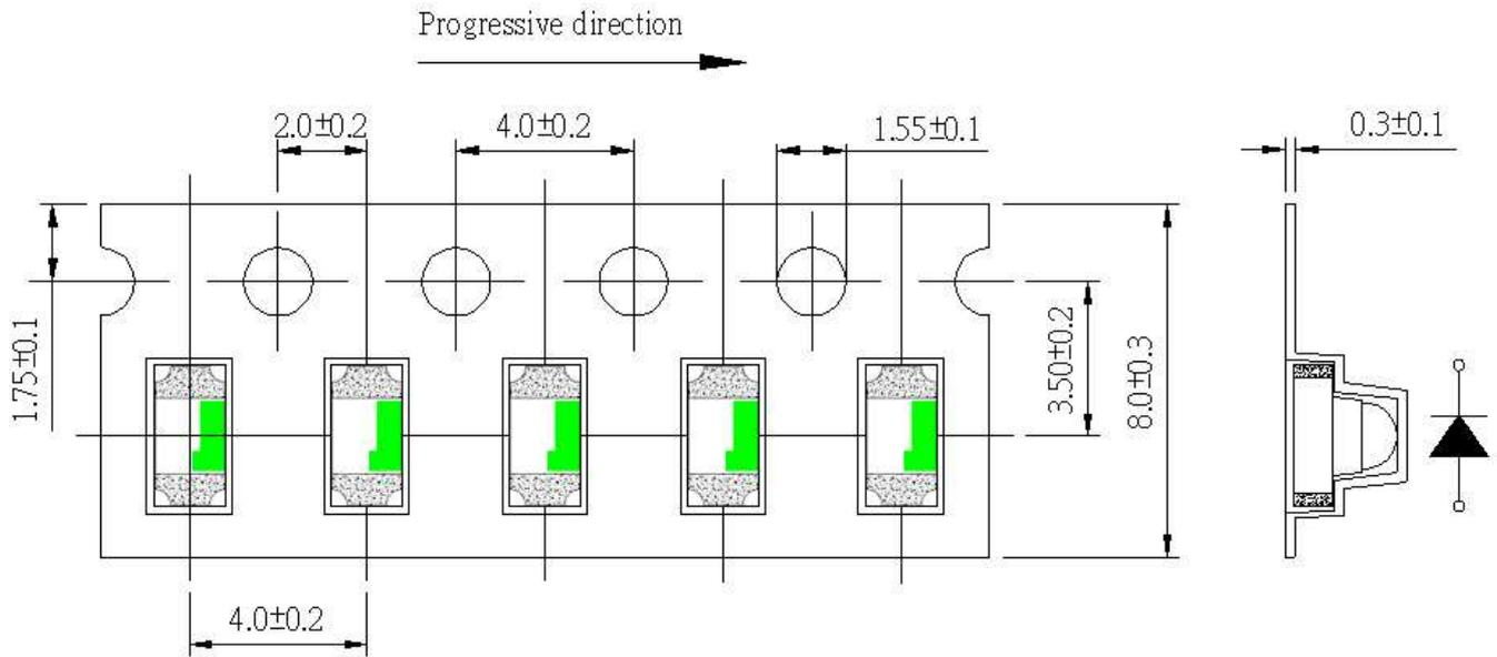
**Note:** Tolerance unless mentioned is  $\pm 0.1$  mm; Unit = mm
