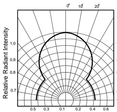
Fig.7 Radiation Diagram(Y-axis)
