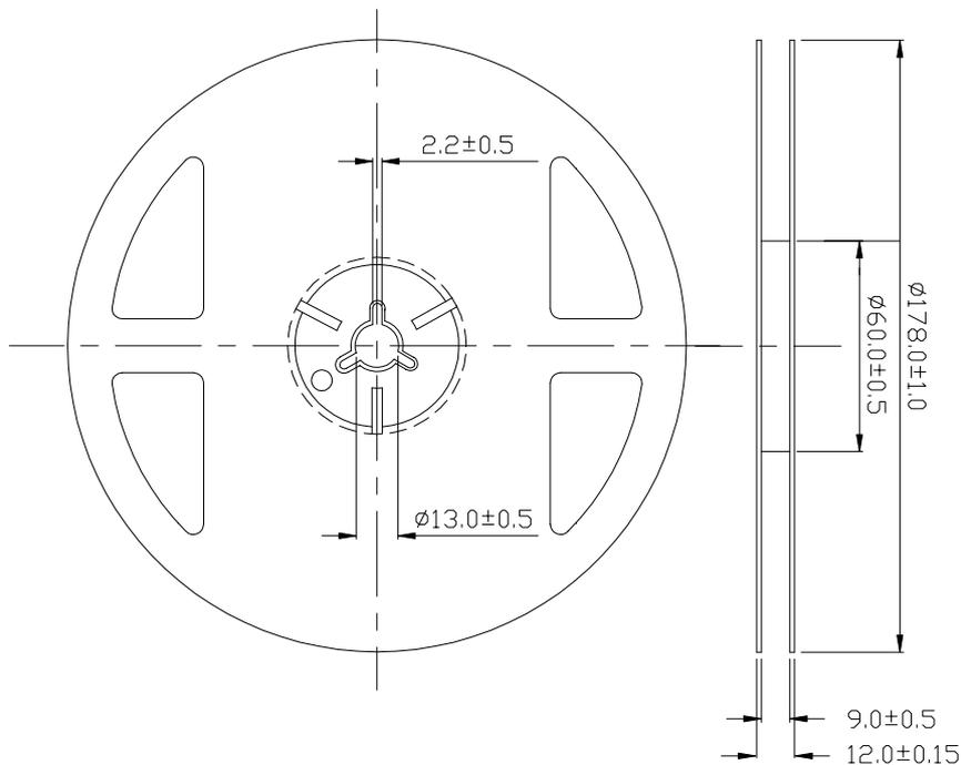
**Note:** Tolerance unless mentioned is  $\pm 0.2\text{mm}$ ; Unit = mm
