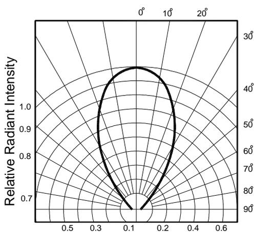
Fig.6 Radiation Diagram (Y-axis)
