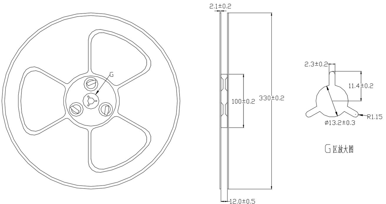
**Note:** Tolerance unless mentioned is  $\pm 0.2\text{mm}$ ; Unit = mm
