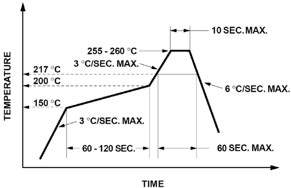
1. Reflow soldering should not be done more than two times.
