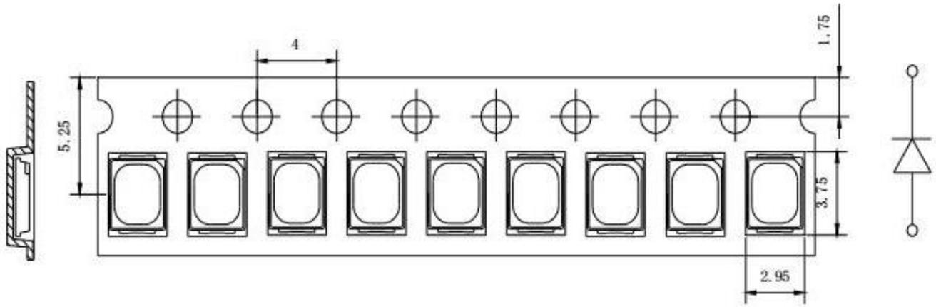
**Note:** Tolerance unless mentioned is  $\pm 0.1$  mm; Unit = mm
