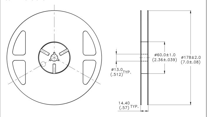
**Note:** Tolerance unless mentioned is  $\pm 0.2$ mm; Unit = mm
