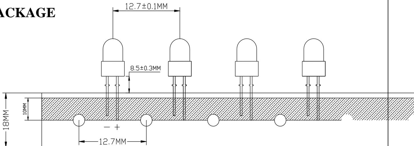
All dimensions are in millimeters. Tolerance is  $\pm 0.20\text{mm}$  unless otherwise noted.
