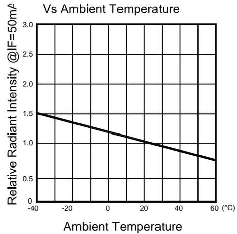
Fig.5 Relative Radiant Intensity
